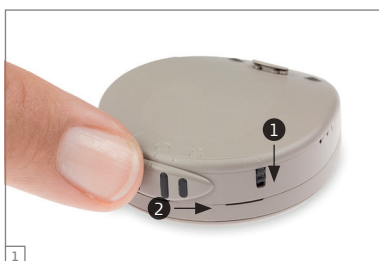
Fig. 16 How to open the battery pack of your RONDO audio processor
