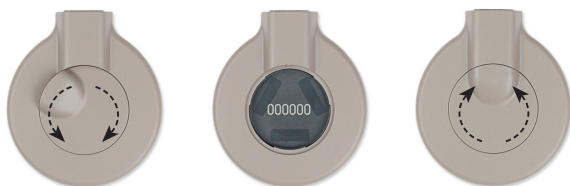
Fig. 10 Removing/inserting the magnet
