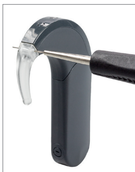
Fig. 17 How to remove the earhook pin
