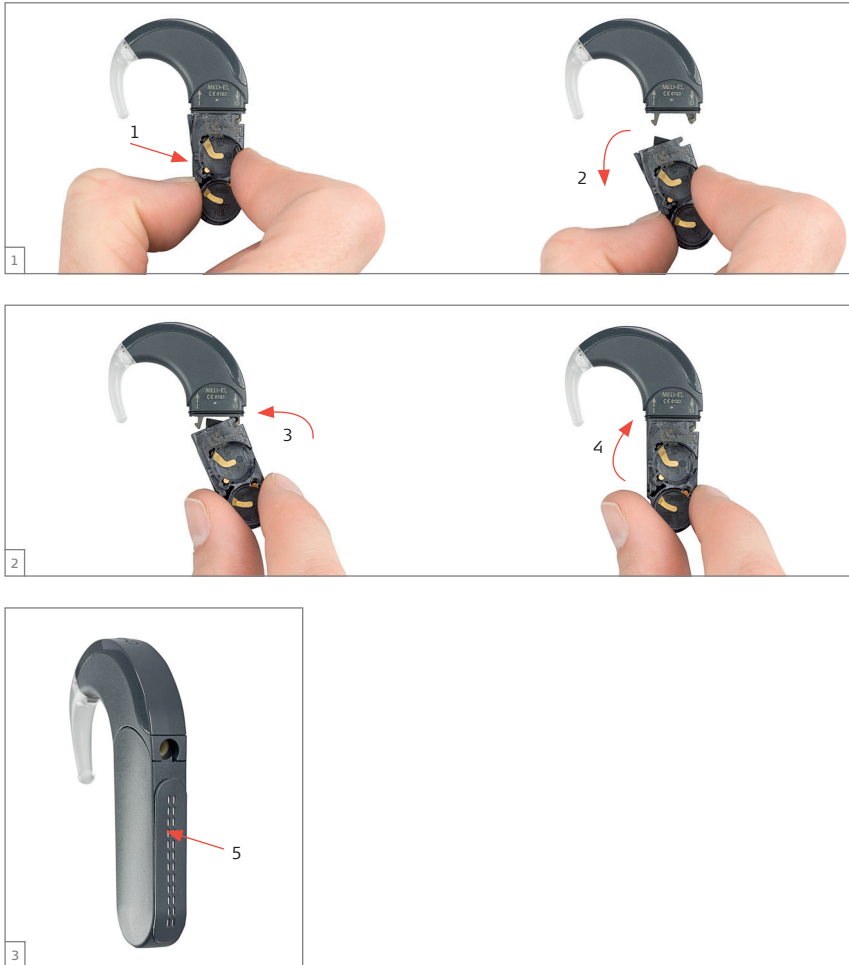
Fig. 8 How to remove/attach the battery pack from/to the control unit
