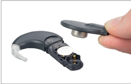
Fig. 22 Changing the batteries of your audio processor
