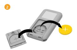
Slide off the battery cover and remove the battery.
