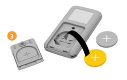
Insert the new battery. Make sure the plus sign "+" is facing up. Take care not to damage the battery contacts.
