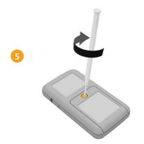
Lock the battery cover in place by turning the screw clockwise with a small Phillips head screwdriver until tight.
