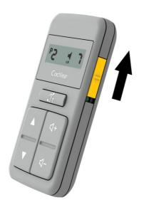
Slide the switch up to turn on.
