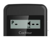
If your processor is out of range or experiencing interference, the remote control displays dashes (shown left).
