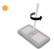
Unlock the battery cover by turning the screw anticlockwise with a small Phillips head (cross-head) screwdriver.
