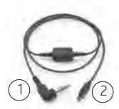
Figure 16: FM listening system end (1) and processor end (2) of the FM Cable
