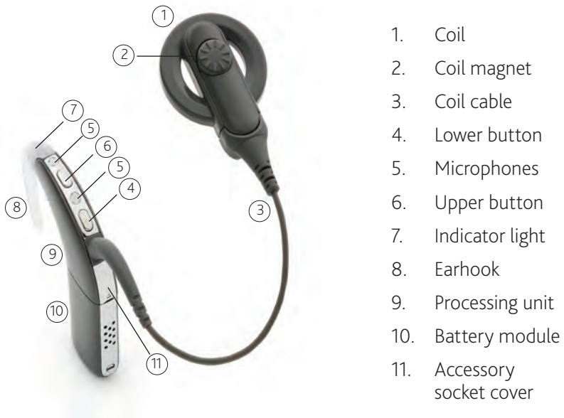
Figure 1: CP810 Sound Processor parts
