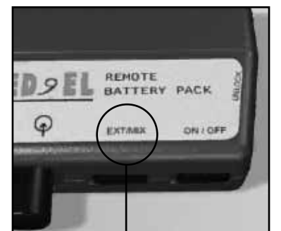
The remote battery pack has the mixing option built into the battery pack
