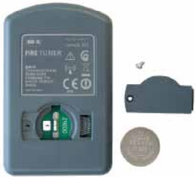
Insert the new battery with the “+” sign facing up.
