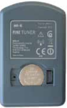
Insert the new battery with the “+” sign facing up.
