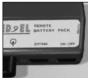
Detail of the input port, EXT/MIX and ON/OFF switches of the remote battery pack.
