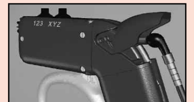
Insert the cable into the socket with the red dot pointing upward. It is not necessary to force the cable in the socket.
