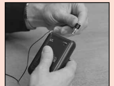
Connect the other end of the cable into the battery-operated device's headphone jack.
