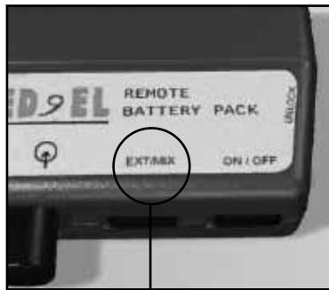
The remote battery pack has the mixing option built into the battery pack
